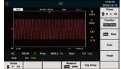
IT7600 series allows users to set their own output fluctuation rate of voltage or frequency, so that the voltage or frequency regularly reach the set value step by step. It is more accurate to verify the product operation scope and also can reduce surge current of DUT when starting up.
