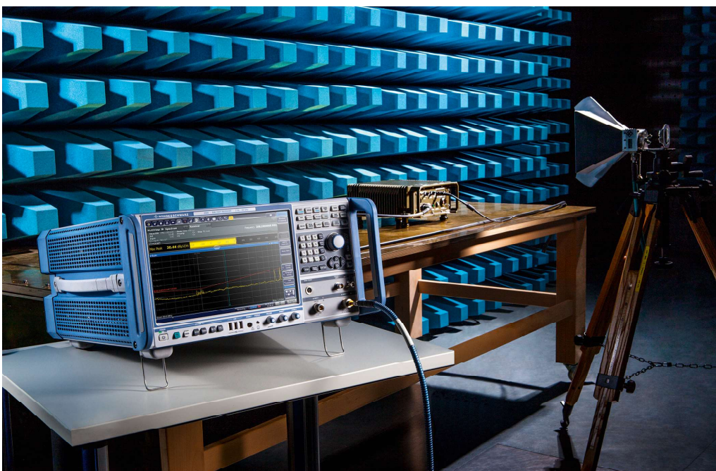
EMI testing in an anechoic chamber.
