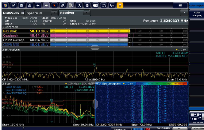
MultiView display with bargraphs, scanned RF spectrum, IF analysis and spectrogram.
