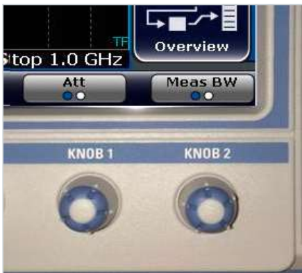
Two rotary knobs with user-assignable functions.
