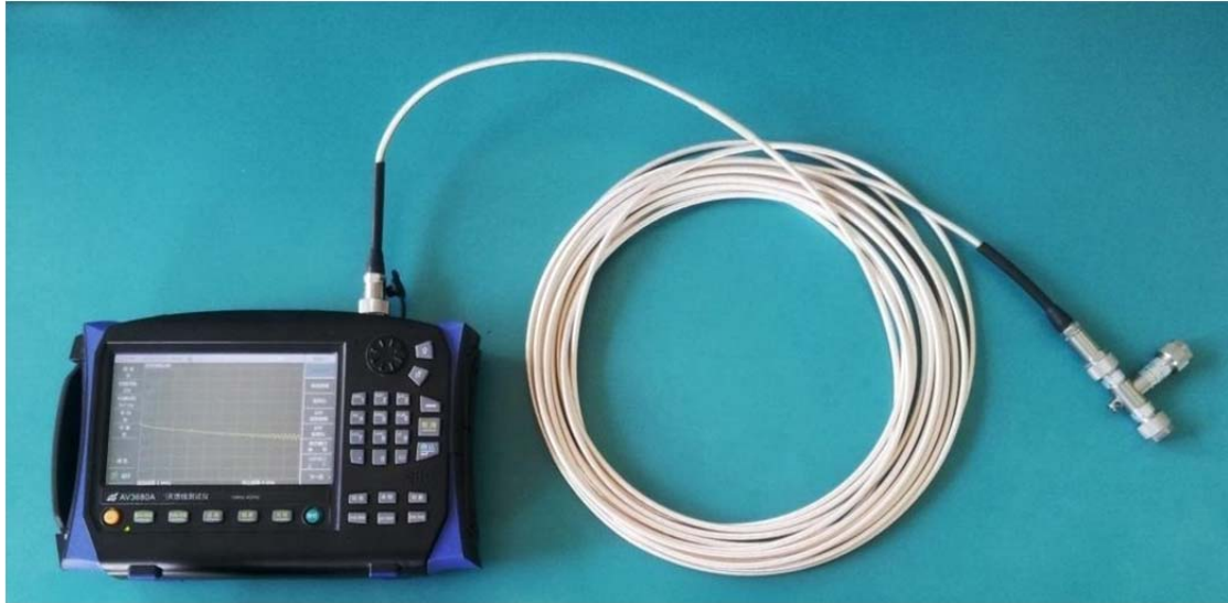
Cable loss measurement
