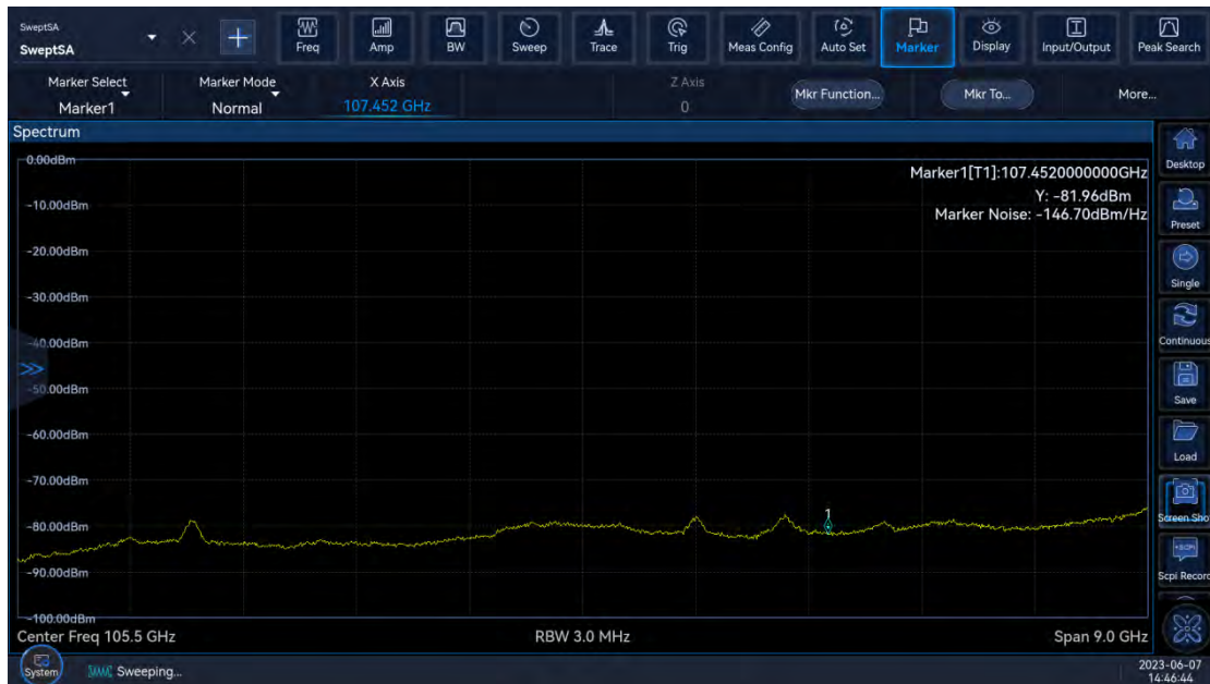
101GHz to 110GHz frequency band DANL specification
