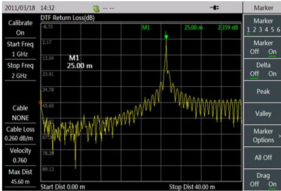
Figure 3.12 Measurement on Length of Cable
