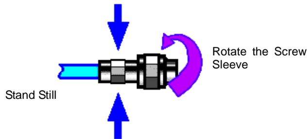
Figure 3.4 Connection Method
