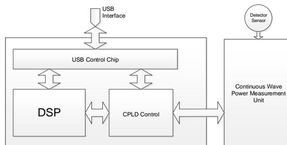
Figure 6.1 Block Diagram of USB Continuous Wave Power Sensor
