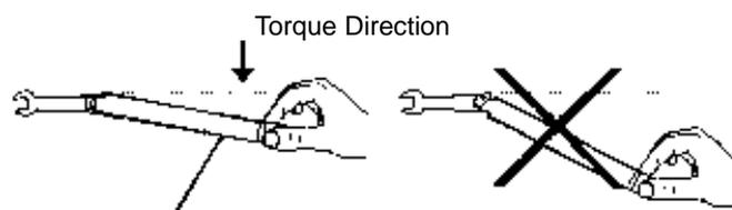
Stop the force when the handle is bent
