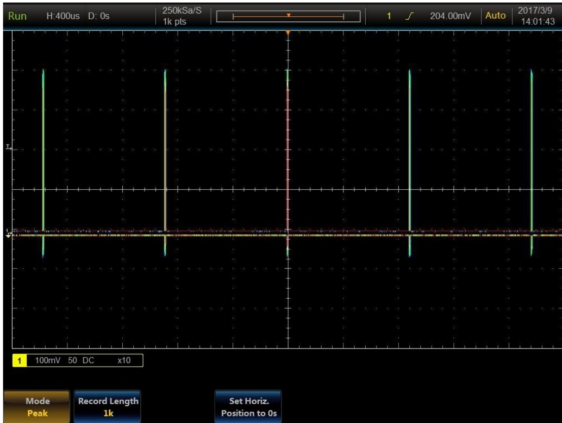
The smallest pulse capture width is 200ps.
