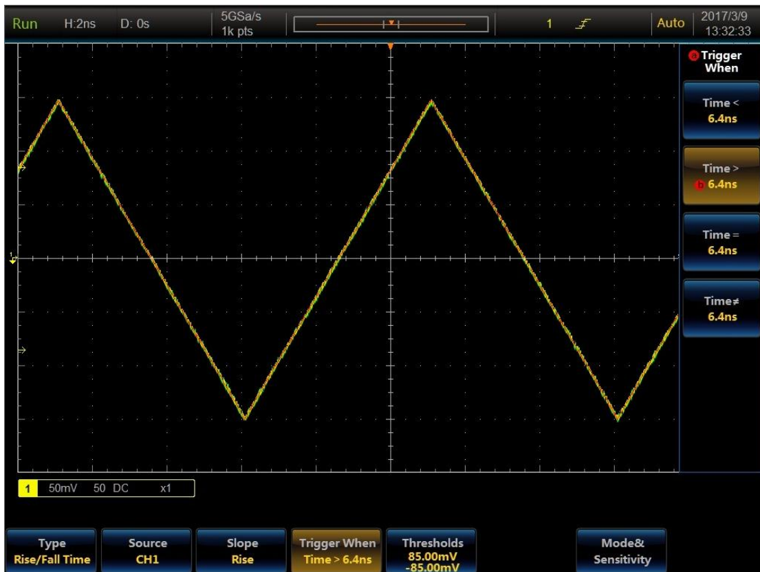
Advanced trigger: runt pulse, logic, sequence, setup and hold time, rise and fall time .
